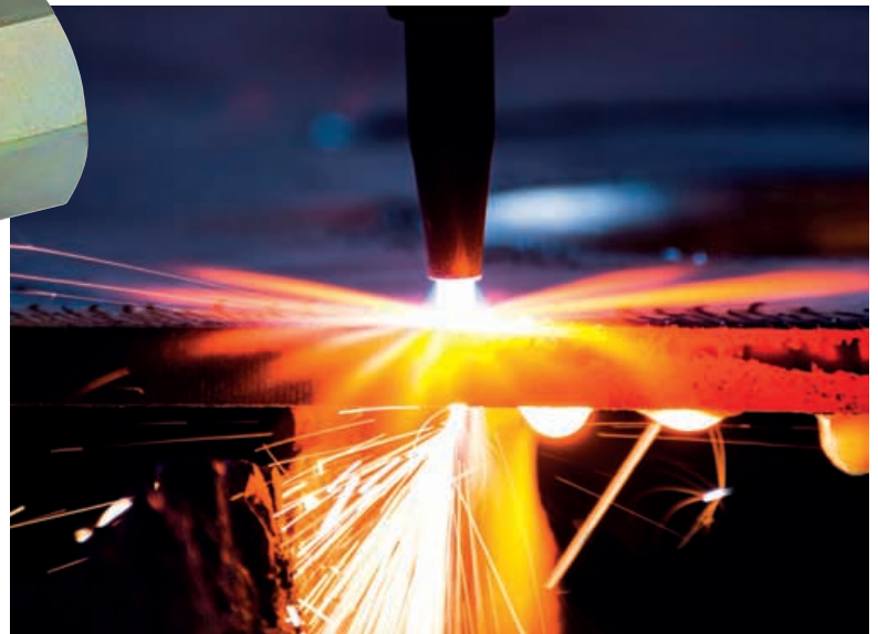
Gas cutting of 50 mm sheet
