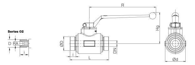
Series 02 (for non-soldering compression fittings with cutting ring DIN 2353, light-duty series)
