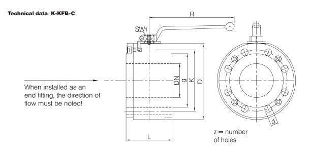
Series 52 (flanges according to ANSI B16.5 Class 600 - Raised Face (RF)
